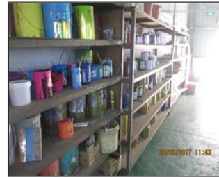
Photo of non-conformity No secondary containers for the chemicals in the silk printing department.JPG
